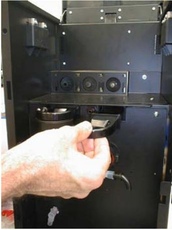
and the aspiration drawers. Immerse all parts in the solution. Using a cloth soaked in the solution, proceed to clean also the attachment bases of the mixers, which remain fixed to the machine. The time of permanence in the solution, in order to obtain a full disinfecting, is stated on the packaging of the chemical.
