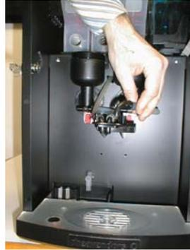
Remove the liquid waste bucket,
