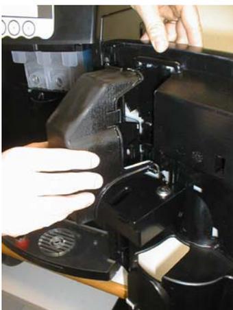
3. Remove the coin-mec protection inside the door;
