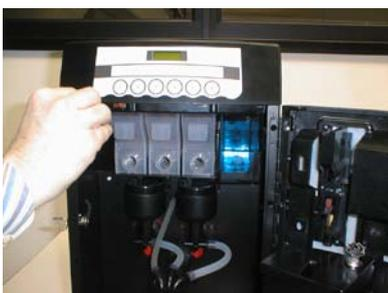
A safety switch is provided in the machine, **which cuts the power off to all 24 V supplied components in the machine when the door is opened.**
