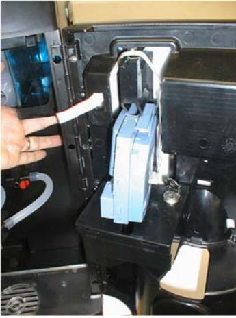
5. Connect the dialogue cable to CPU board on the rear side of the machine;
