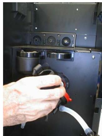
remove the pipes support, remove the mixing bowls, the mixing fan.
