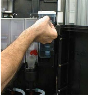
Fill the internal independent water tank using drinking water. If it is necessary demand a laboratory certification to a specific analysis laboratory. To fill in water, lift the water refilling cover or extract the tank from the machine and pour drinking water inside the tank. The capacity of this tank is about 2 litres.
