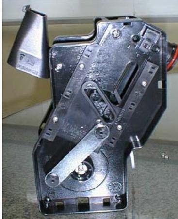
Turn the group in the position of ejection waste grounds and overturn the slide of coffee
