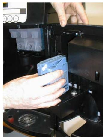
4. Fit the coin-mechanism;
