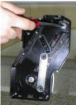
Remove the plates of the superior filter
